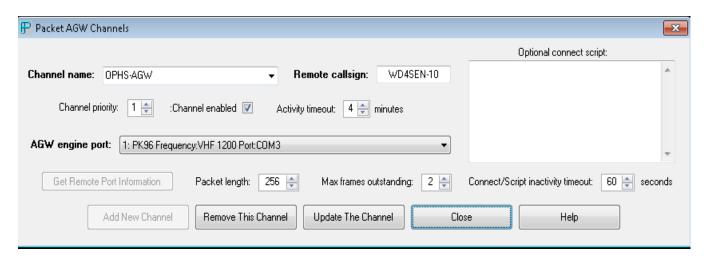
Step 4B - Configure Packlink to communicate with TNC Directly
