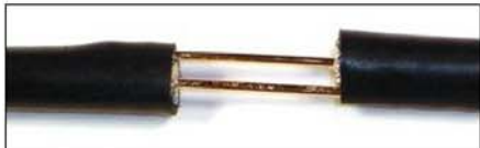
Figure 5 — Continue twisting the two pieces together, keeping the two center conductors parallel.
