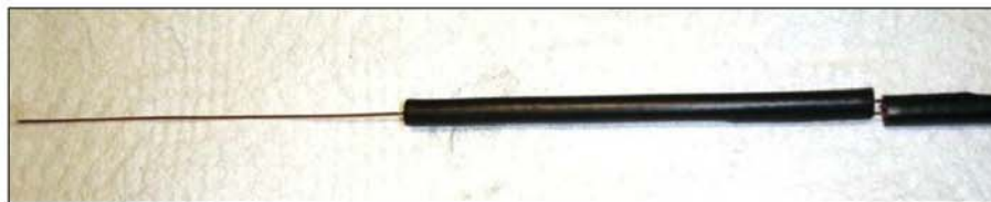
Figure 7 — Top section of the antenna with the 4\frac{1}{2} inch exposed center conductor acting as a vertical element.
