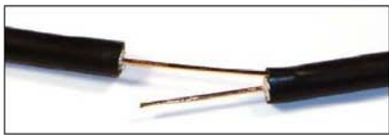
Figure 4 — Assembly is eased by heating the outer jacket either in an oven or with a heat gun. Pinch the outer covering to create a small gap and then first insert the longer exposed conductor between the outer jacket and the foil shield. Next insert the shorter exposed conductor and slide the two pieces together using an alternating twisting motion.
