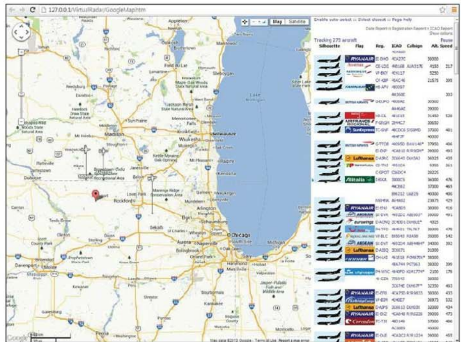
Figure 2 — Real time aircraft tracking using Virtual Radar Server software with aircraft positions plotted on Google Maps.
